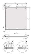
U-profile front panel for textile EMC gasket.
