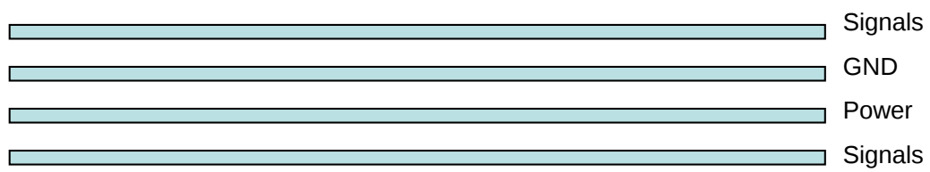
Figure 8: Typical 4-layer PCB construction
