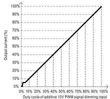
Note: 1. Min. dimming level is about 8% and the output current is not defined when 0%< Iout<8%.
