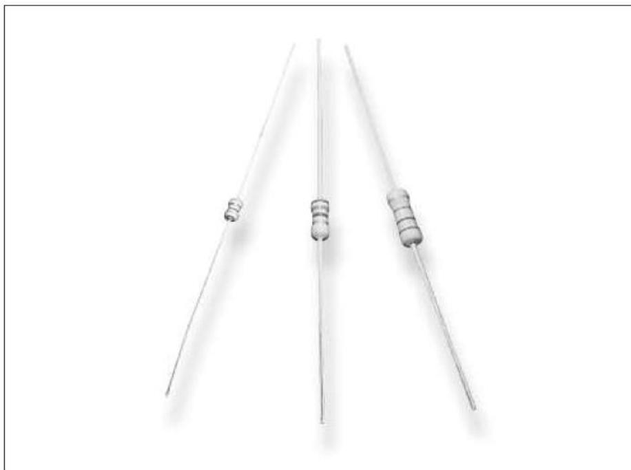
The resistive element comprises a thin film of carbon, deposited onto a high thermal conductivity ceramic core. Metal end caps are force fitted to the element prior to spiralling to value. Tinned copper lead wires are welded to the end caps and the components are then coated. One coat of phenolic resin is followed by three coats of epoxy resin. All resistors are tested for value and tolerance.
