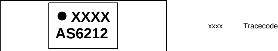
Figure 14: WLCSP package marking/code for AS6212
