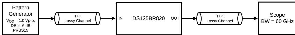
Figure 10. Test Setup Connections Diagram
