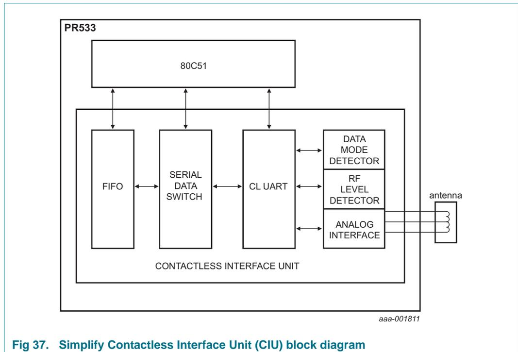
The Analog Interface handles the modulation and demodulation of the analog signals according Reader/Writer mode communication scheme.
