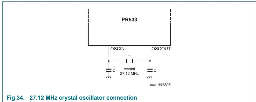
Fig 34. 27.12 MHz crystal oscillator connection
