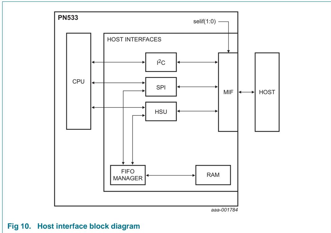
Fig 10. Host interface block diagram
