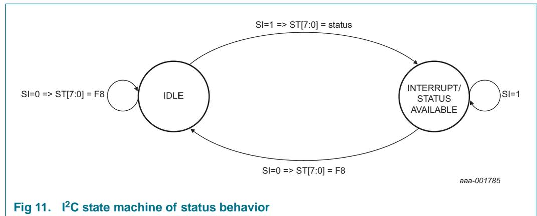
Fig 11. I<sup>2</sup>C state machine of status behavior
