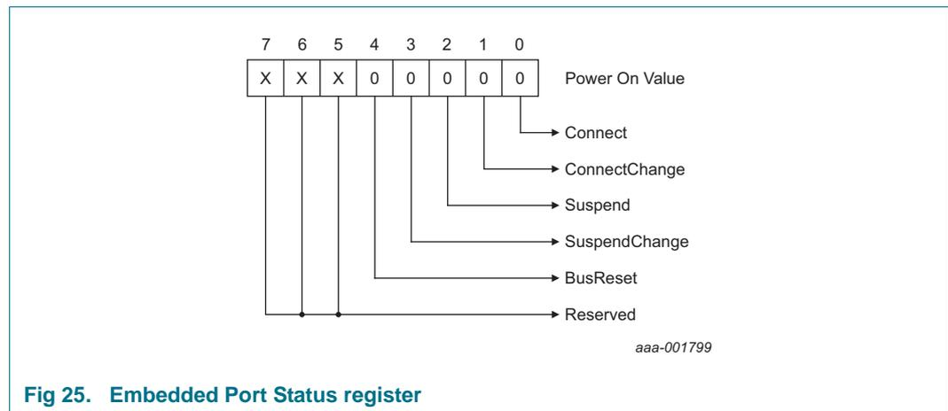
**Fig 25. Embedded Port Status register**
