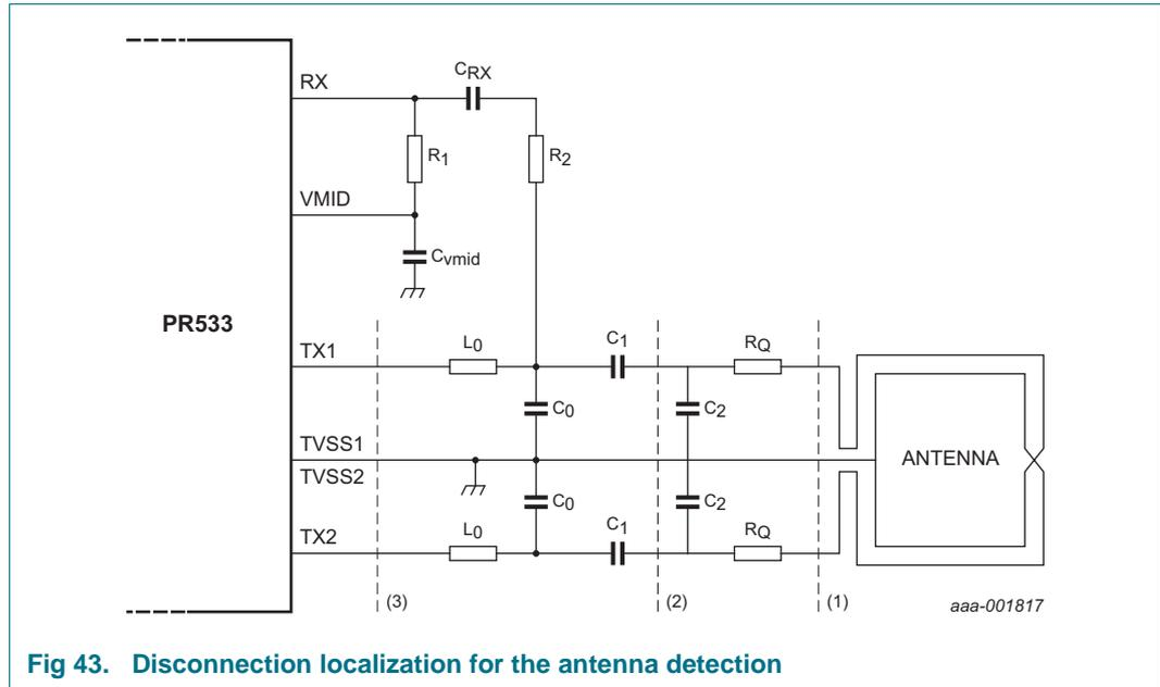
Fig 43. Disconnection localization for the antenna detection
