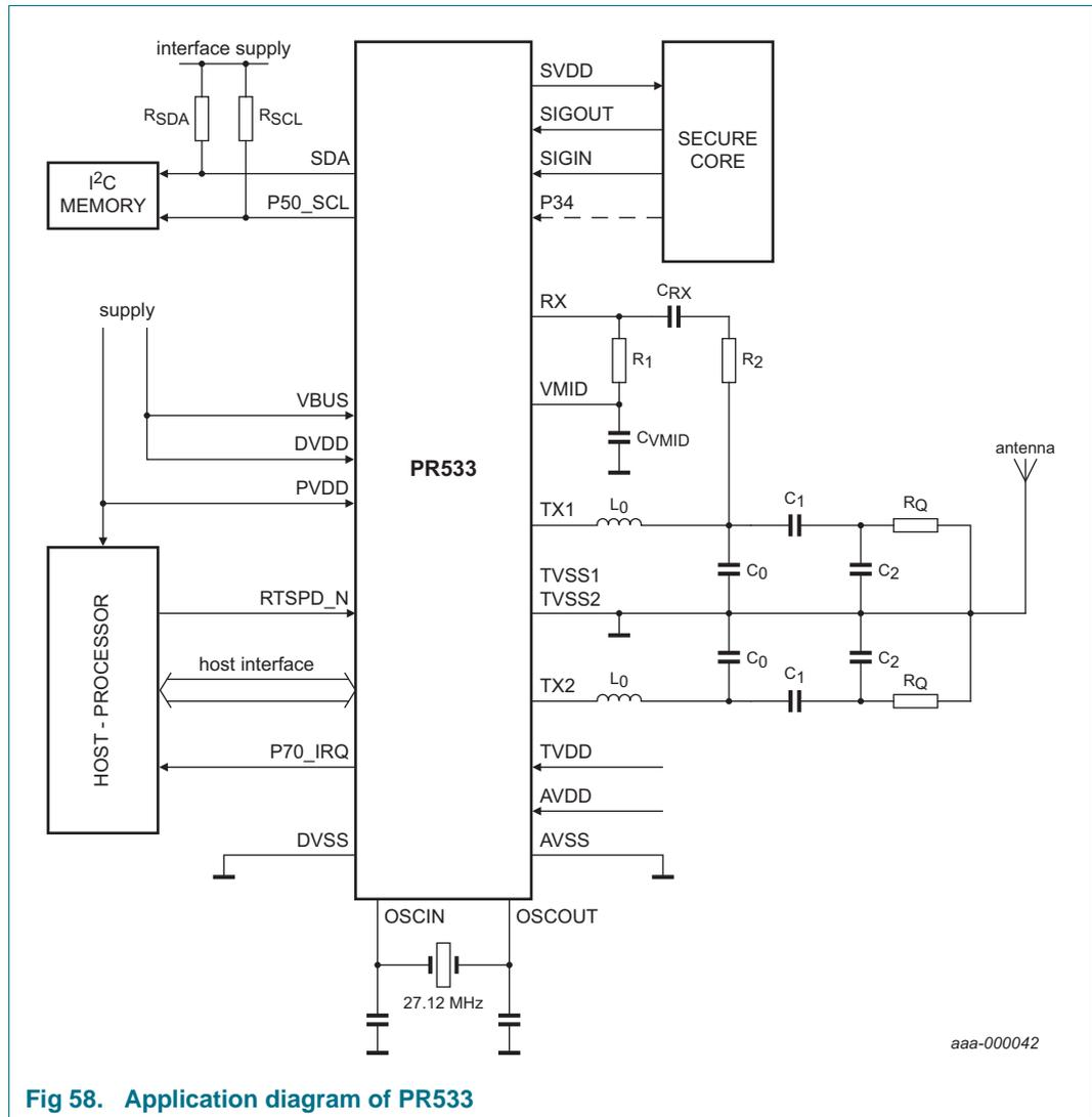
Fig 58. Application diagram of PR533
