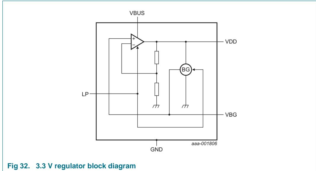
Fig 32. 3.3 V regulator block diagram
