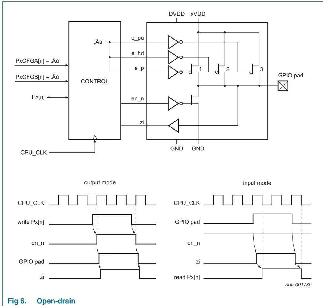
Fig 6. Open-drain
