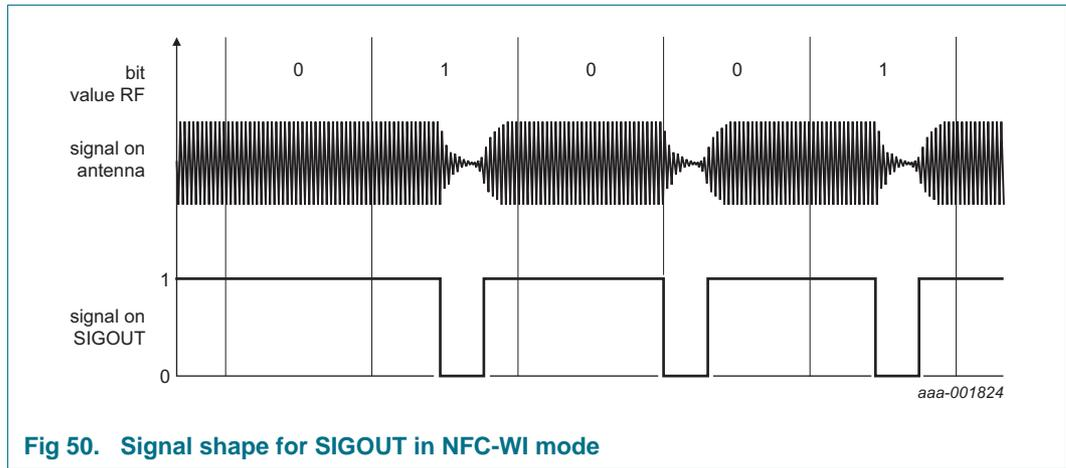
**Fig 50. Signal shape for SIGOUT in NFC-WI mode**
