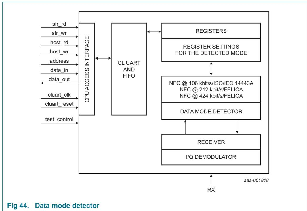
Fig 44. Data mode detector
