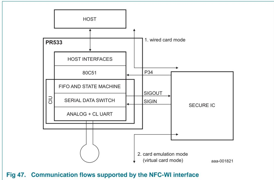
**Fig 47. Communication flows supported by the NFC-WI interface**
