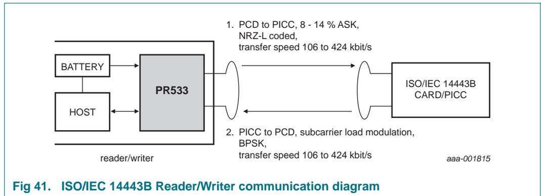
**Fig 41. ISO/IEC 14443B Reader/Writer communication diagram**
