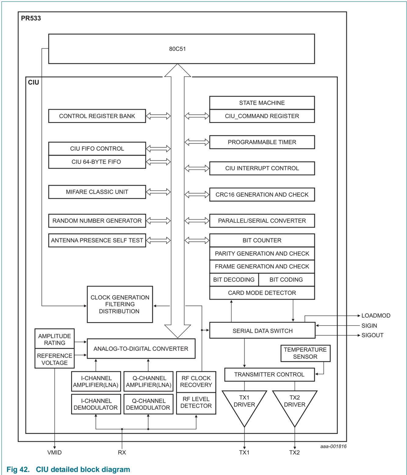
Fig 42. CIU detailed block diagram
