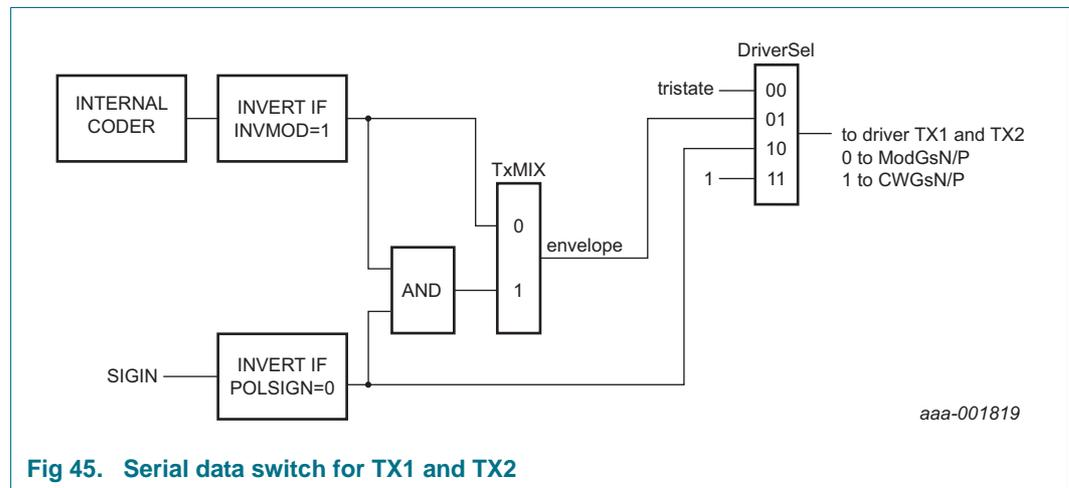
**Fig 45. Serial data switch for TX1 and TX2**
