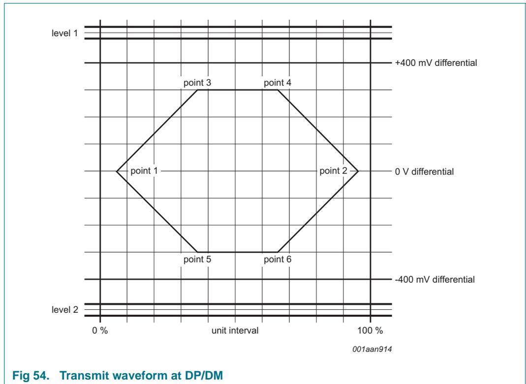
**Fig 54. Transmit waveform at DP/DM**
