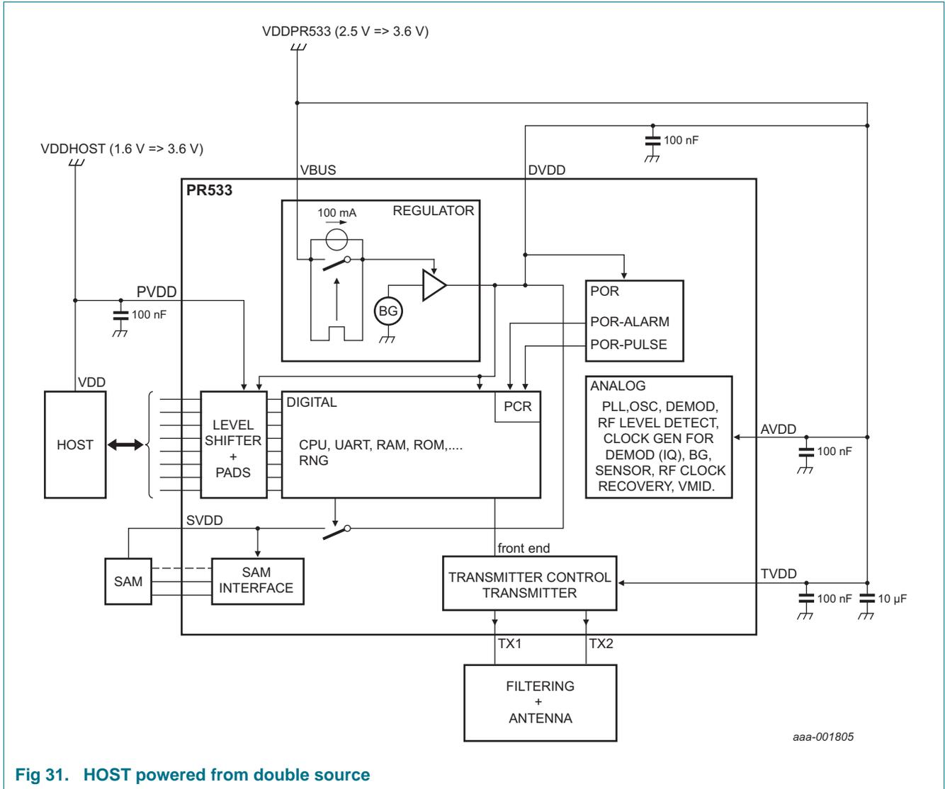
Fig 31. HOST powered from double source
