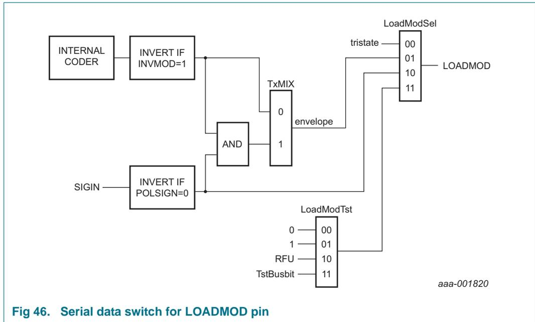
Fig 46. Serial data switch for LOADMOD pin
