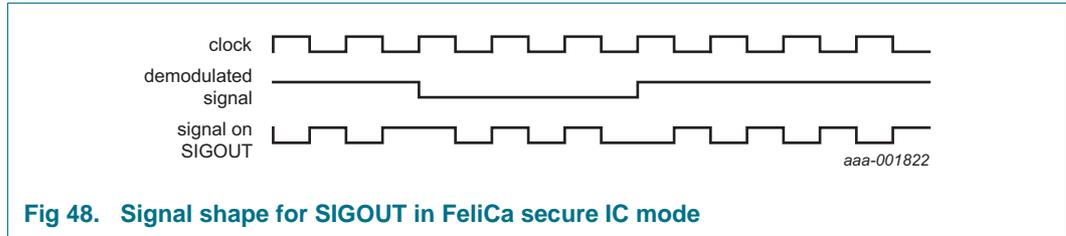
**Fig 48. Signal shape for SIGOUT in FeliCa secure IC mode**
