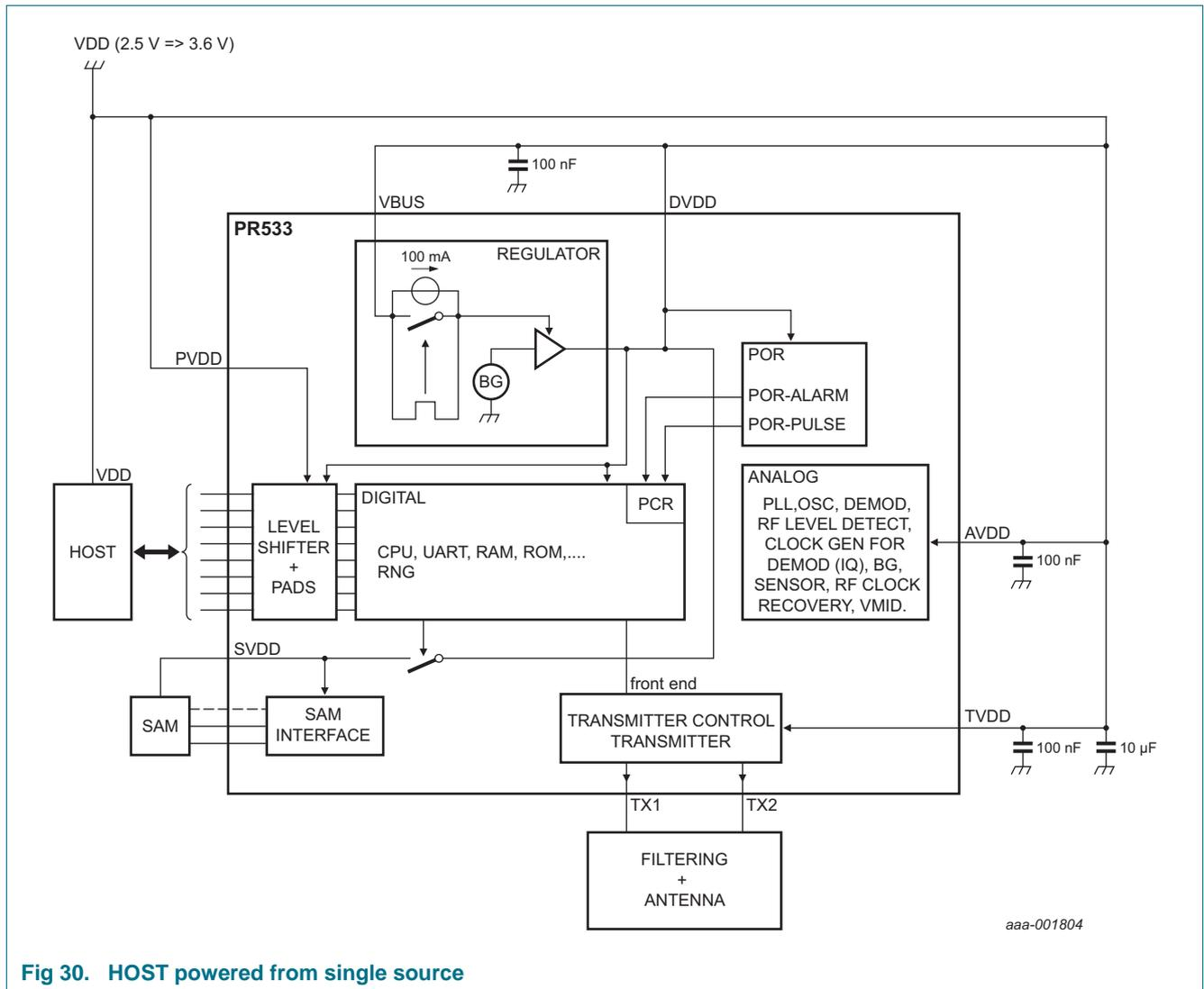
Fig 30. HOST powered from single source
