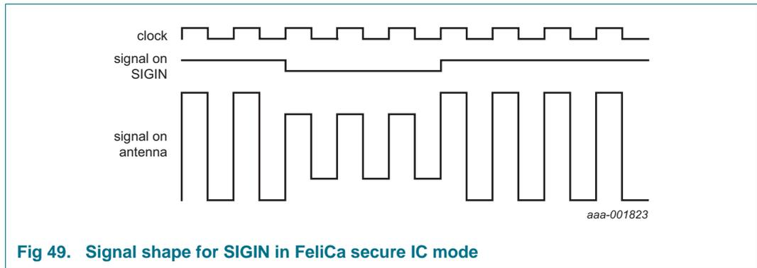
**Fig 49. Signal shape for SIGIN in FeliCa secure IC mode**
