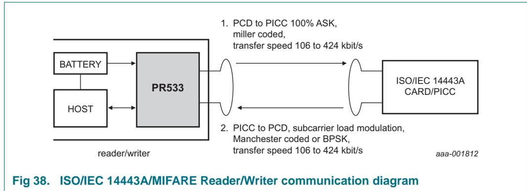
**Fig 38. ISO/IEC 14443A/MIFARE Reader/Writer communication diagram**
