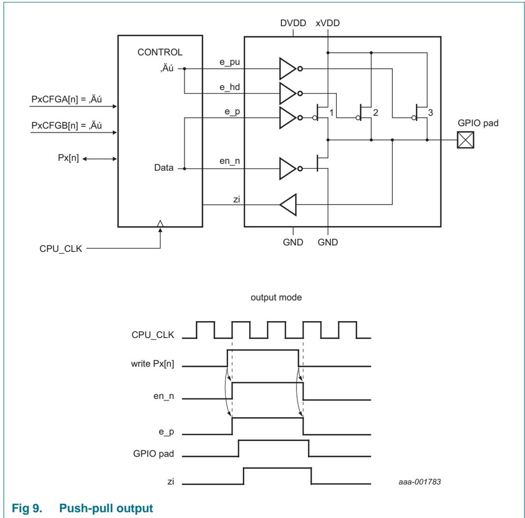
Fig 9. Push-pull output
