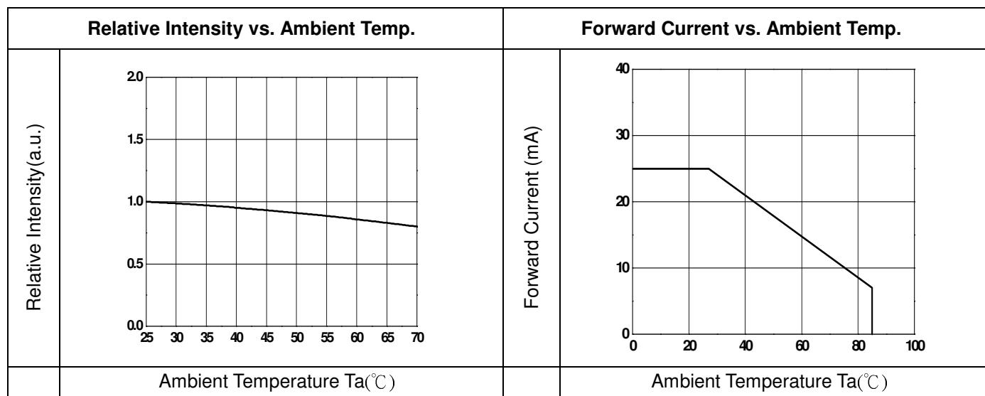
**Typical Electro-Optical Characteristics Curves
