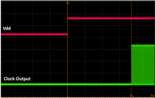
Figure 16. Startup Waveform vs. Vdd
