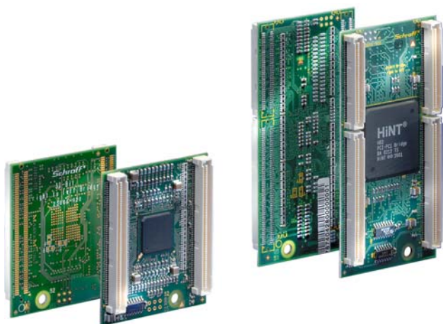
Photo shows 32-bit and 64-bit bridges
