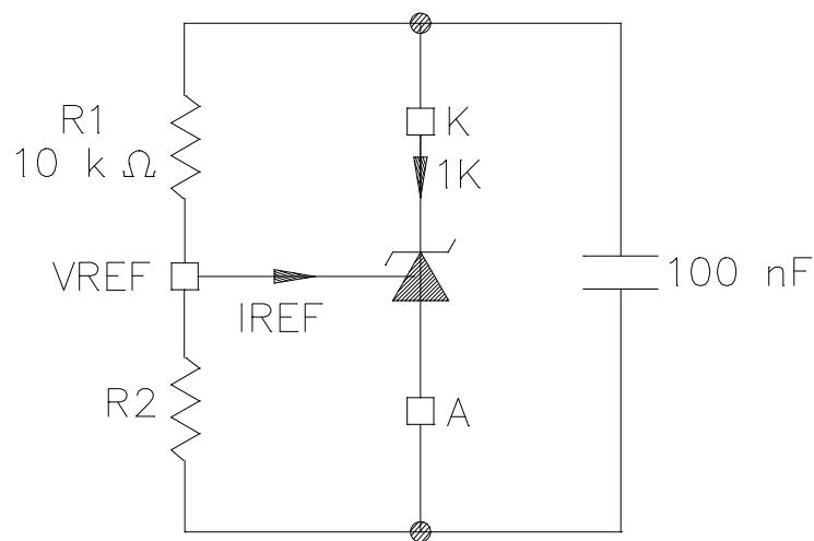
FIGURE 3. Cathode to anode voltage test circuit.
