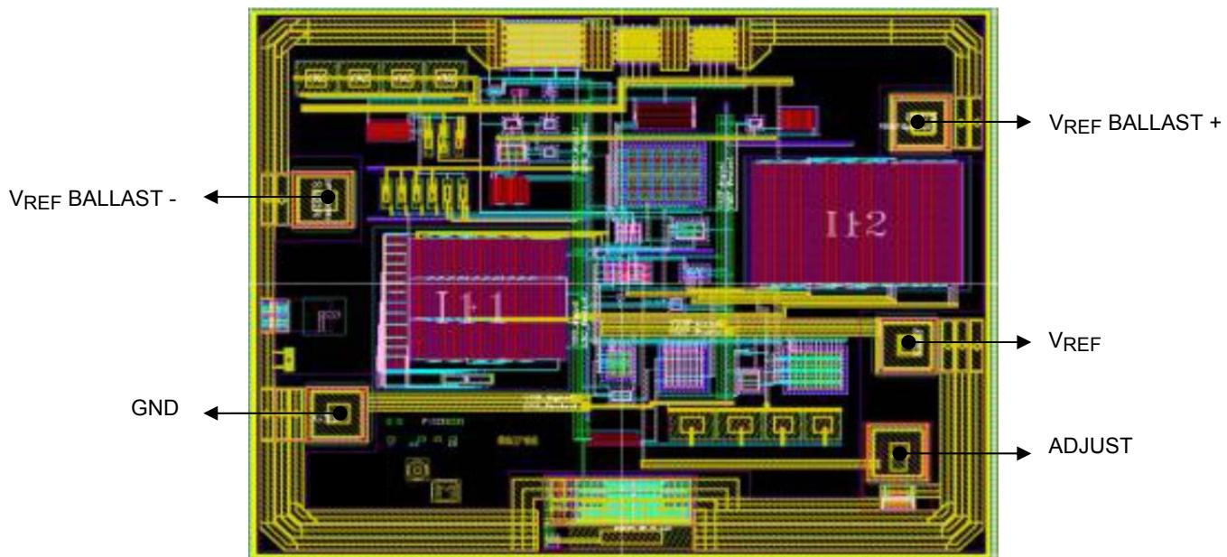
FIGURE A-1. Die bonding pad locations and electrical functions.
