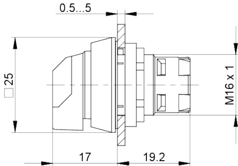
**Mounting hole drawing**
