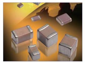
AVX's M123 series MIL-qualified ceramic capacitors are designed for high performance application in BX voltage temperature characteristics for general purpose dielectric and in BP voltage temperature characteristics for temperature stable dielectric.
