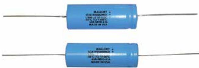
Type TCX is an axial leaded, 105 °C, 2000 h extended life industrial and computer grade quality aluminum electrolytic capacitor with low DCL and ESR and is suitable for computer applications.
