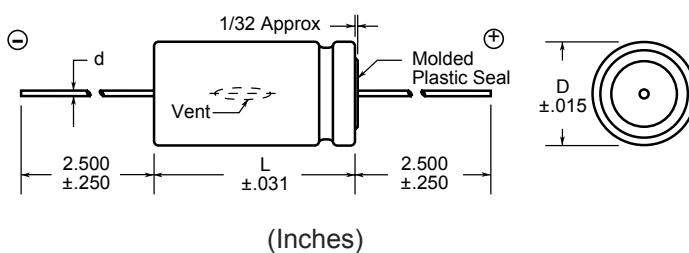
Parts are supplied with PVC insulating sleeve.
