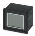
Touch panel with 7.1 cm/2.8" TFT-display (analog resistive (polyester)), 320 x 240 pixel(s) (QVGA), 4 colors, Cortex™-M3 120 MHz, without, 1 x Ethernet (10/100 Mbps), RJ45, Keil RTX (RTOS) and user software: PC Worx. (bus system: without)
