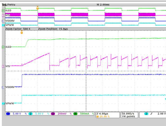
Ch1: DDRV voltage; Ch2: PWM input; Ch3: Switch sense current resistor voltage; Ch4: LED current; Time: 4 \mu s/div
