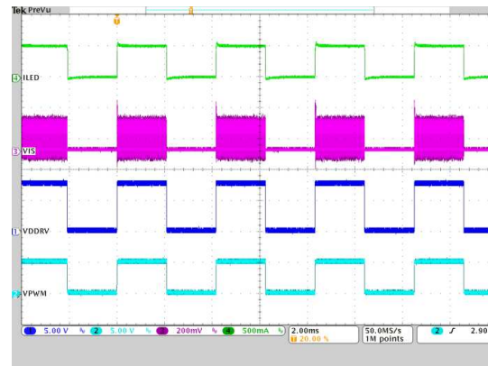
Ch1: DDRV voltage; Ch2: PWM input; Ch3: Switch sense current resistor voltage; Ch4: LED current; Time: 2 ms/div
