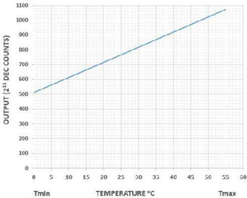
$$\text{OUTPUT (DECIMAL COUNTS)} = \frac{(\text{OUTPUT}^{\circ}\text{C} + 50^{\circ}\text{C}) \times 2048}{150^{\circ}\text{C} - (-50^{\circ}\text{C})}$$
