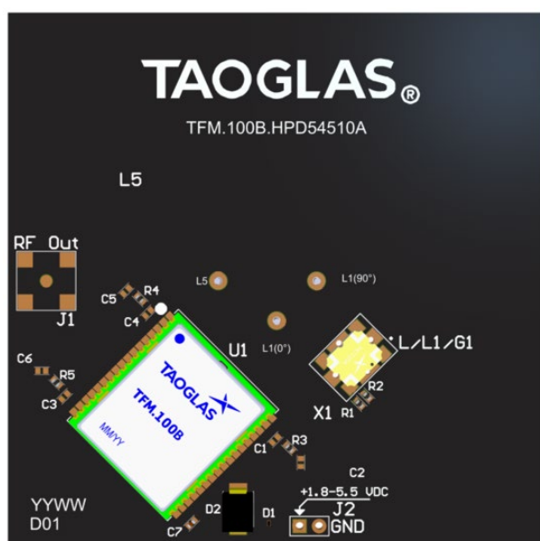
Bottom side (TFM.100B placement including HC125A )
