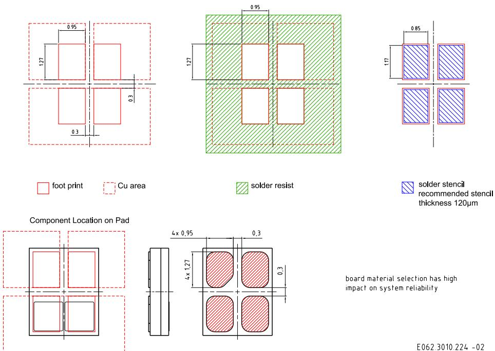
For superior solder joint connectivity results we recommend soldering under standard nitrogen atmosphere. Package not suitable for ultra sonic cleaning. To ensure a high solder joint reliability and to minimize the risk of solder joint cracks, the customer is responsible to evaluate the combination of PCB board and solder paste material for his application.
