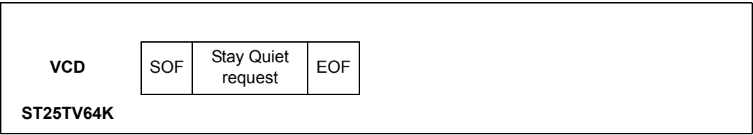
Figure 41. Stay Quiet frame exchange between VCD and ST25TV64K
