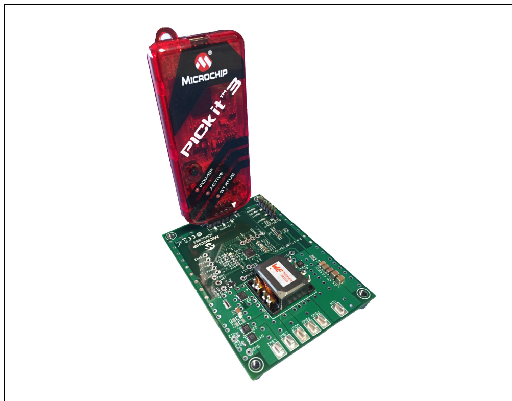
FIGURE 2-3: PICkit 3 In-Circuit Debugger/Programmer Connected to the MCP19117 Flyback Stand-Alone Evaluation Board.
