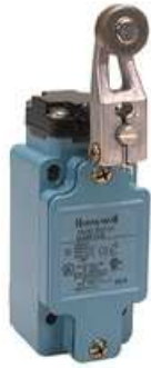
Global Limit Switches Series GLS: Side Rotary With Rod - Adjustable, 2NC 2NO DPDT Snap Action, 0.5 in - 14NPT conduit
