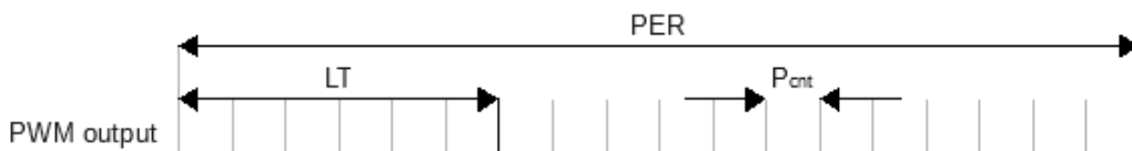
Figure 59 – Simple PWM with POL = 1
