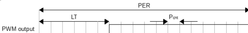
Figure 58 – Simple PWM with POL = 0
