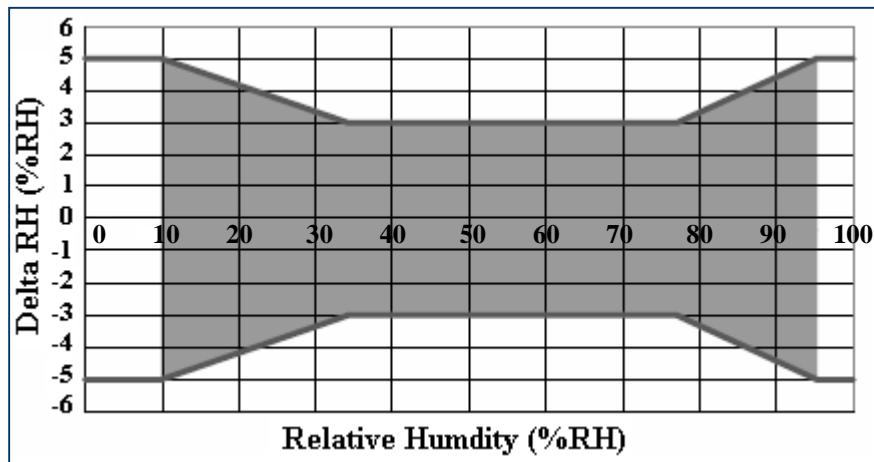
HTG3500 series modules are specified for maximum accuracy measurements within 10 to 95 %RH.
