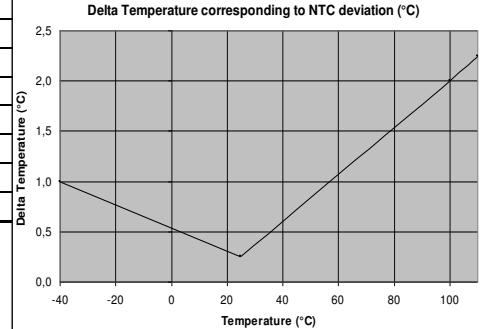
0.1°C tolerance on Resistance Measurement
