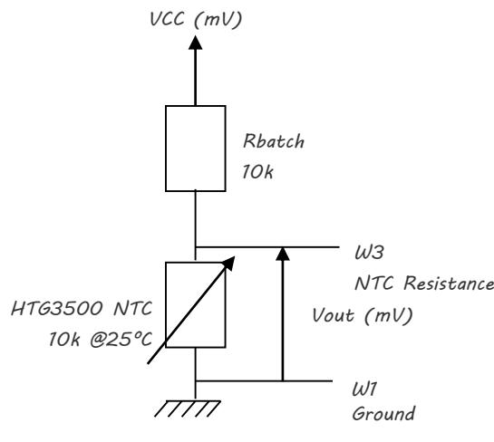
$$V_{out}(mV) = \frac{V_{cc}(mV) * NTC_{HTG3500}(\Omega)}{R_{batch}(\Omega) + NTC_{HTG3500}(\Omega)}$$
