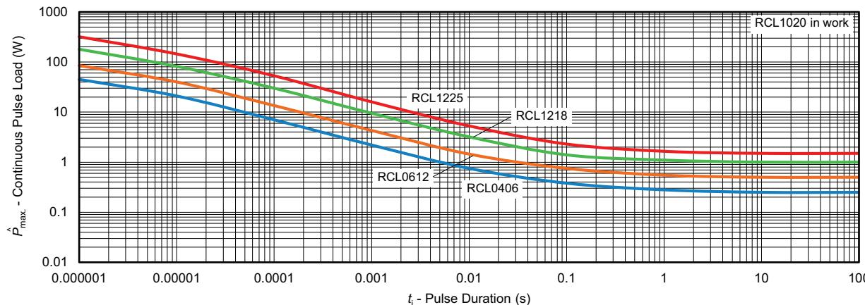
Maximum pulse load, continuous pulses; applicable if  $\bar{P} \leq P(v_{\text{amb}})$  and  $\hat{U} \leq \hat{U}_{\max}$ ;
