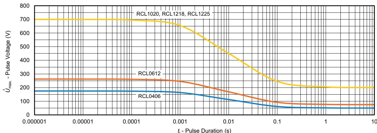
Maximum pulse voltage, single and continuous pulses; applicable if  $\hat{P} \leq \hat{P}_{\max}$ ;
