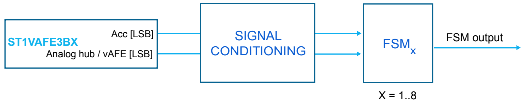
Figure 16. State machine in the ST1VAFE3BX
