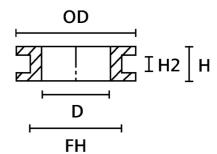
Material: Polyvinylchloride, flame retardant (PVC-
