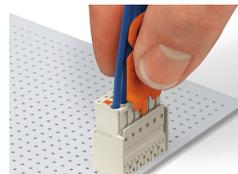
Pull on both unlocking tool and conduc-
