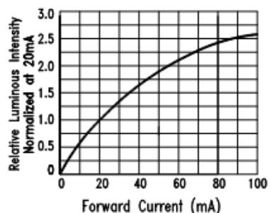
Fig.4 Relative Luminous Intensity
