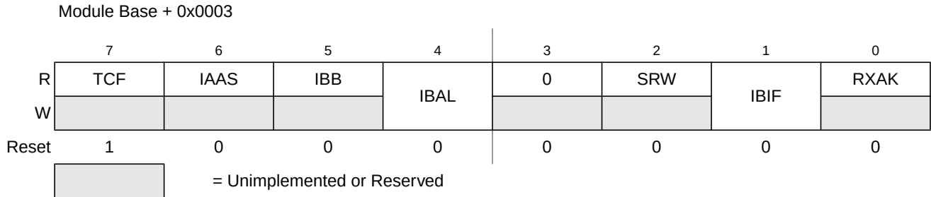
Figure 10-7. IIC Bus Status Register (IBSR)
