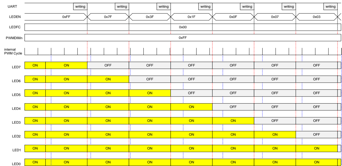
Figure 40. Sequential Winker 2 (Sequential LED OFF) LEDEN Controlled
