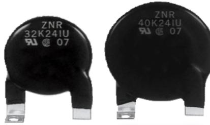
Varistors (ZNR Surge Absorber) with Tabs is a heavy duty type ZNR with very unique tab terminals which bring forth a higher reliability. These tabs are used as electrical connecting terminals and also its mounting legs. This type of ZNR is meant for applications in power supplies or transient voltage surge suppressor units where large surge current or high surge energy absorption is required.
