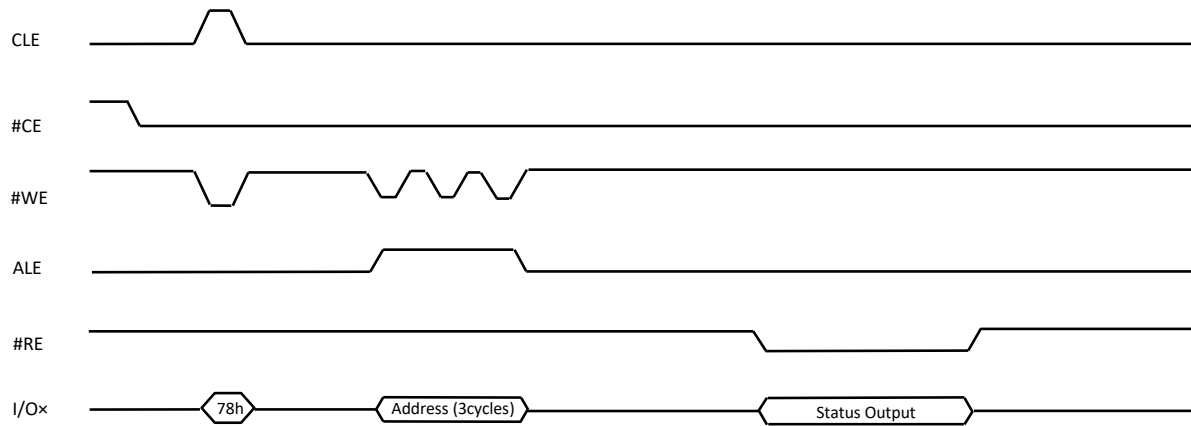
Figure 9-8 Read Status Enhanced (78h) Operation
