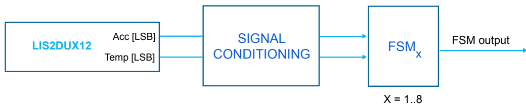
Figure 11. State machine in the LIS2DUX12
