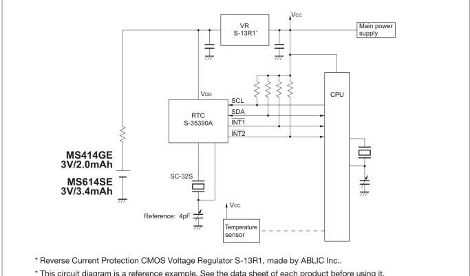
\* This circuit diagram is a reference example. See the data sheet of each product before using it.
