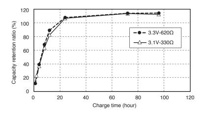
Both the MS621T and MS920T can reach 80% of capacity after 12 hours of charging.
