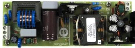
In addition, the controller includes a new high voltage circuitry that combines a start-up current source and a brown-out detector able to sense the input voltage either from the rectified ac line or the dc filtered bulk voltage. The high voltage sensing circuitry is used for the overpower protection purposes as well. Overpower protection, overload protection, and next protective features increases the safety level of the final application.
