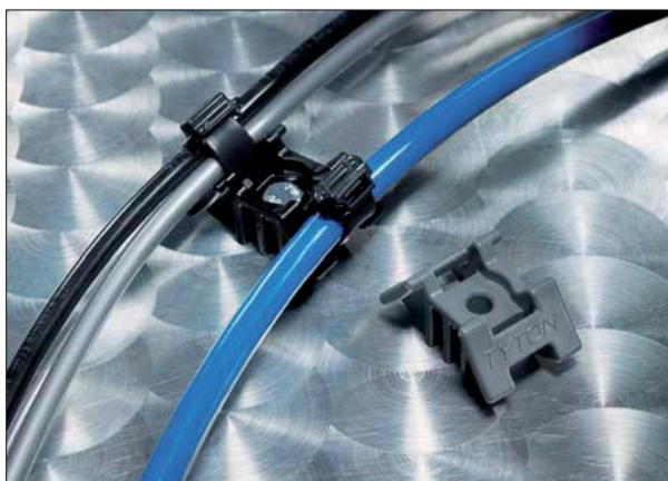
This saddle mount is installed between two bundles to separate them and prevent chafing and wear.
