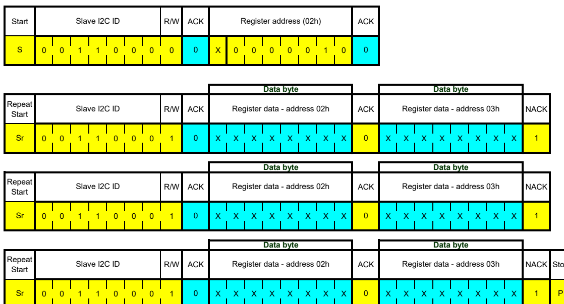
Figure 41: Multiple read transmissions of I 2 C from the same start address
