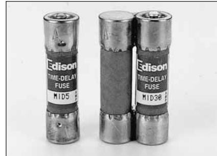
Catalog No. MID (0.1 - 30A) 0.1 - 0.8A 250Vac or Less 1 - 15A 125Vac or Less 20 - 30A 32Vac or Less Pin Indicating - Time-Delay
