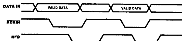
Figure 21. Interlocked Handshake Timing (Input) Port 2 Side Only
