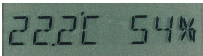
Figure 21. Temperature and Humidity Display
