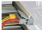
Testing with test plug modules.
