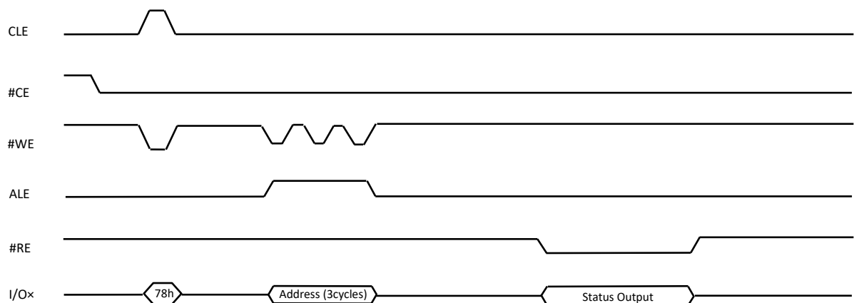
Figure 9-7 Read Status Enhanced (78h) Operation
