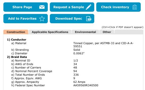
Alpha braid is an exceptional, low resistance way to create a point-to-point ground strap. In retrofit applications, braid is an ideal way to install additional shielding to your cable.
