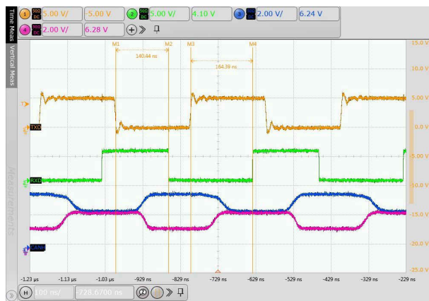
Figure 8-16. Typical TXD, RXD, CANH and CANL Waveforms at 5 Mbps
