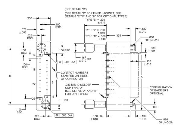
FIGURE 1. Connectors, plug, .100 (2.54 mm) spacing.
