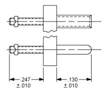
TYPE "X" FULL ROUND GUIDE PIN AND SOCKET DETAIL F
