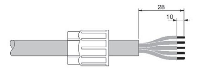
Strip 28 mm off the cable, 35 mm in the case of the angled version, strip single wires, push the pressure nut onto the cable. Slide the wires through the sleeve housing and connect, screw sleeve housing to the plug insert, screw the pressure nut tight.
