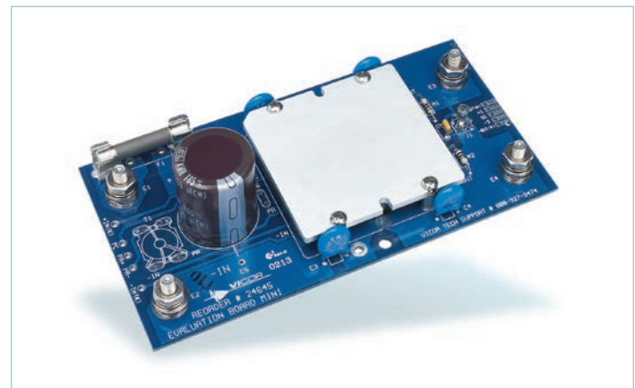
Figure 2.15 — Evaluation Boards; Available for Maxi, Mini and Micro Family DC-DC converters
