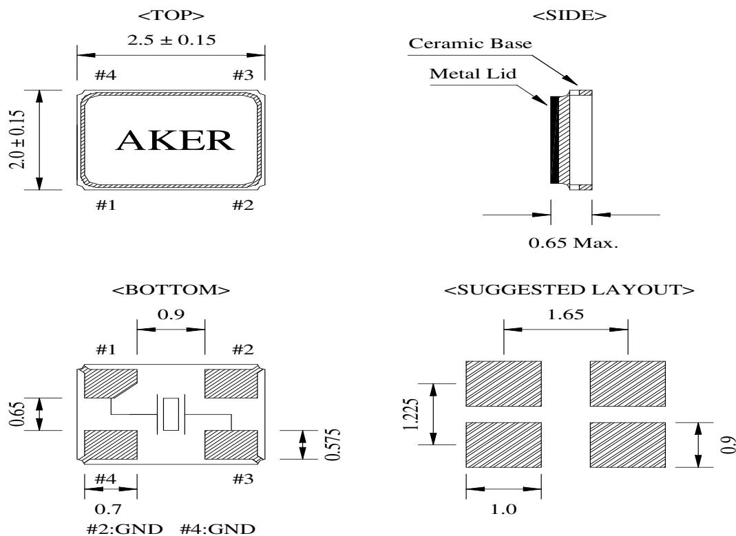
Package is Seam Sealed Ceramic-Metal.
