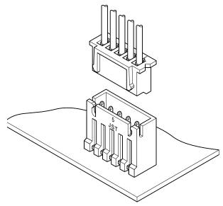
XH connector high box type, with 17.0 mm mounting height and with 5.8 mm thickness.
